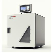
The Ahiba IR moves the beakers in a circular rotation with advanced infrared heating technology that eliminates glycol contamination and cumbersome beaker cleaning. The specially designed pressure tested beakers offer maximum safety and can be used for atmospheric and high temperature dyeing. Chemical auxiliaries can be easily added through our specially designed beaker lid without removing the lid.
