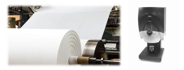
Datacolor ELREPHO, a trusted spectrophotometer for the paper industry, suitable for the reference laboratory or production control of color, brightness, opacity, diffuse reflectance factors, yellowness, and whiteness of pulp, paper and chemicals. It uses a diffuse/0 optical geometry and automated, adjustable, ISO 2469 compliant UV filter.
