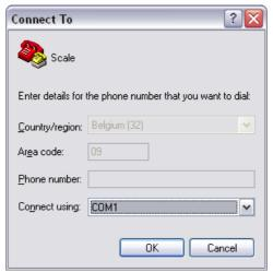
Connect with the communication parameters set correctly (baudrate,databits,parity,handshake). These parameters have to be the same as on the scale. This picture is only an example.
