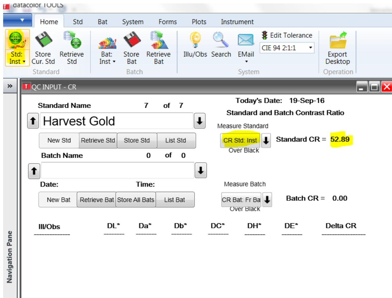
The sample placed at the aperture plate of the spectro and backed up by a white background. The Standard measurement button, Std Inst, in Home ribbon bar above was used for this measurement. The white background was then replaced with a black background and a measurement was taken of the same spot on the standard using the button embedded in screen form, CR Std:Inst. The Contrast Ratio then was display as Standard CR = 52.89.
