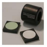
The black trap and white tile are used each time the instrument is calibrated. The green tile is used to perform an optional diagnostic test.
