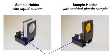
Thumb screws provide the ability to adapt the holder to samples of varying thickness. • The sample holder is mounted onto the transmission sample holder base
