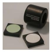
The black trap and white tile are used each time the instrument is calibrated. The green tile is used to perform an optional diagnostic test. If you are using an instrument with an adjustable UV filter, a fluorescent calibration standard will also be included.
