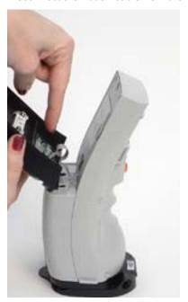
4. On the right side of the battery, there is a black switch. Press this switch down to release the battery.
