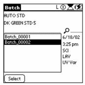
Place the sample at the instrument port and press the Measure button. The program will autoname the batch, and select the appropriate standard for it:
