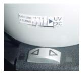
During the fluorescent tile calibration, you may be instructed to adjust the position of this filter. The program will prompt you to turn the Allen Key clockwise, or counterclockwise to adjust the position of the filter:
