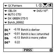
6. To override the measurement sequence, press the **Measure/Select Batch button** on the Control Panel. The screen below displays:
