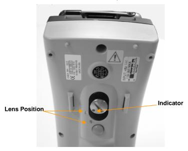
The positions are identified with a letter indicating the lens position (L, S, U). Using a small round disc (a washer or coin will work), turn the switch to the position that matches the aperture size you want to use. The dot on the switch indicates the current position.
