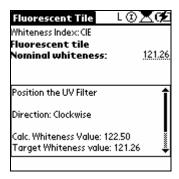
This screen displays the whiteness value for the fluorescent tile, based on the measurement just completed, and instructions regarding the adjustment of the UV filter.
