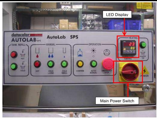
Step 1: Turn on the main power switch, and the "LED Display" will illuminate.
