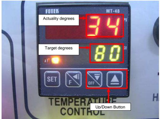
Step 3: Make sure target temperature on controller is correct. If not, change it by following steps 4 to 6.
