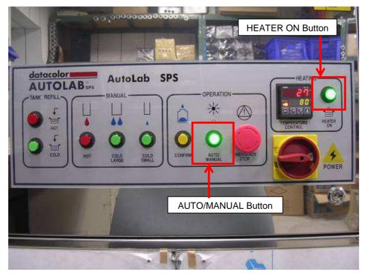
Step 2: Check if the "AUTO/MANUAL" button is on, if not, press it to switch it on.
