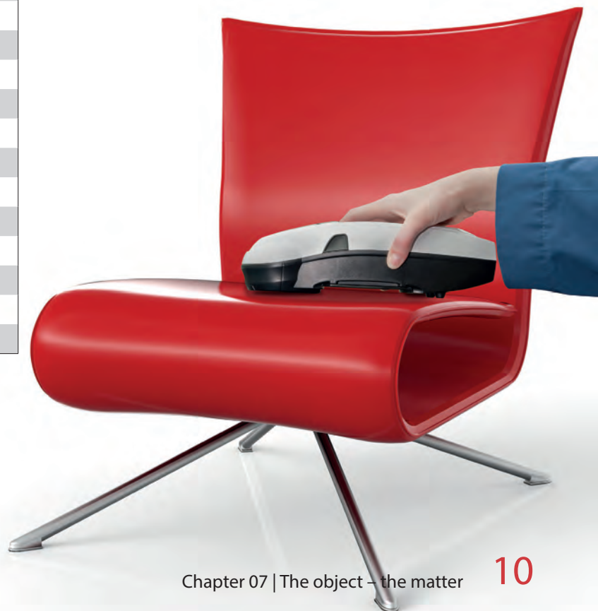
Shiny red sample: measurement with a measurement geometry of d/8° with specularly reflected light (gloss)
