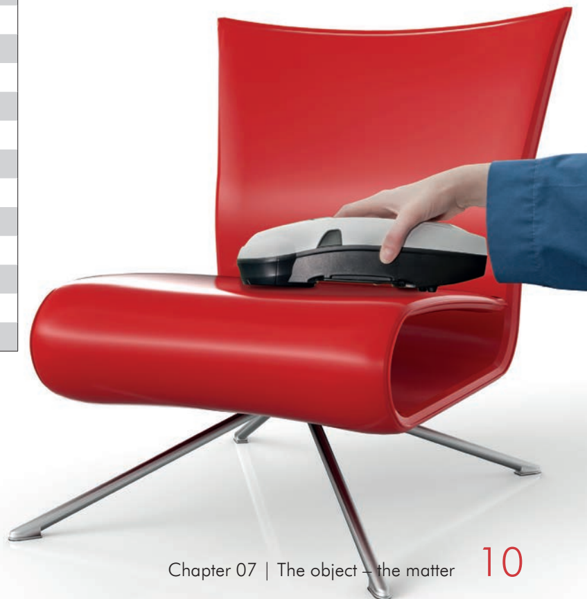
Shiny red sample: measurement with a measurement geometry of d/8^\circ with specularly reflected light (gloss)
