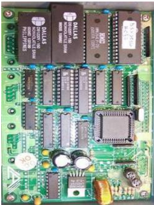
Inner layout of original LA50B CPU (LA600)
